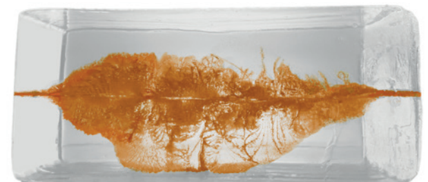
Simulated wound cavity in ballistic gelatin
