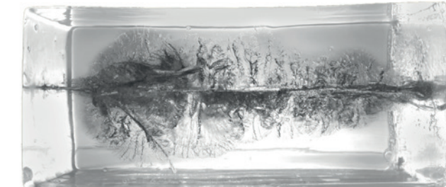
Simulated wound cavity in ballistic gelatin
