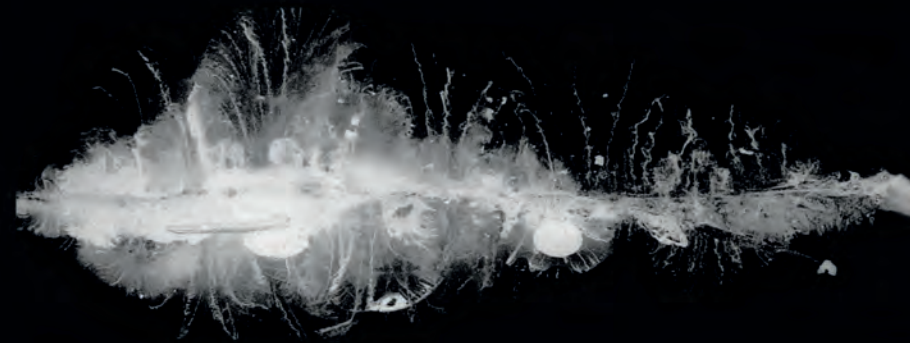
Simulated wound cavity in gelatin block / bullet performance in gelatin
